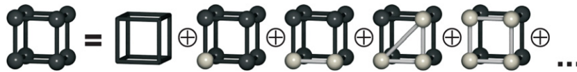
Figure 1. Illustration of the decomposition of a simple cubic lattice into the figures used in the CE. The sum has been truncated with respect to the number of vertices and possible shapes and orientations of figures with the same number of vertices.
