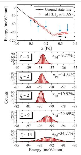
Figure 5. Predicted energies of L1<sub>2</sub>-based antisite structures and their distribution at various concentrations.  $\zeta$  indicates the approximate distance to the ground-state line (in meV/atom) at the corresponding concentrations.
