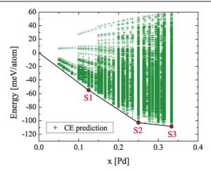
**Figure 3.** Ground-state diagram in the Cu-rich regime. Each triangle represents the predicted energy for one specific crystal structure. The solid line is the convex hull of all  $\mathcal{O}(10^6)$  energies. The ground-state structures are depicted in figure 2. L1<sub>2</sub> is not a ground state, but rather the L1<sub>2</sub>-related superstructure S2 (LPS 3).
