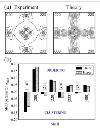
**Figure 4.** (a) Experimental [5] versus theoretical short-range order for  $Cu_{0.702}Pd_{0.298}$  at T=773 K in reciprocal space. The SRO exhibits peaks of the fundamental wavevector  $\mathbf{k}=(1,1/2M,0)$  at M=3, in excellent agreement with the superstructure period of S2. (b) Real space SRO for neighbouring pairs separated by [lmn].
